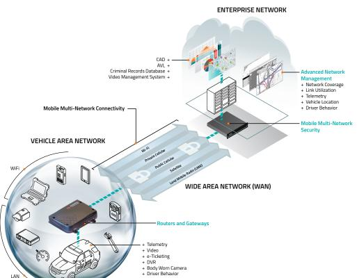
Connection Manager (ACM), the MG90 consolidates the security for all connected technologies in the vehicle area network (VAN), vastly simplifying deployment and enabling the enterprise to retain management control over network access and connected mobile assets.
